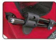
7 Extend the side bars by pressing down the side locks on both sides of the frame and flip down the locks to secure both steel bars together.
