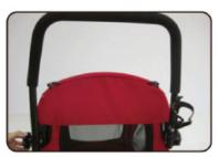
6 Turn the hand screw on both sides of the handle to lock it securely to the frame.
