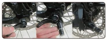
8 Steps 8 to 11 are for bike trailer use only. Securely install the towing receptacle on the rear wheel axel as the picture shown
