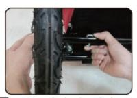
1 Content: 1Trailer frame / container, 1 Insert rear wheel axel into the frame receiver till it clicks, press the lock to allow proper locking. Check both wheels are securely locked by pulling. It might be necessary to disengage the foot brake.
